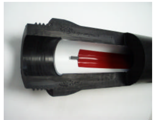
Igniter wire installed on the inside of an M grain
