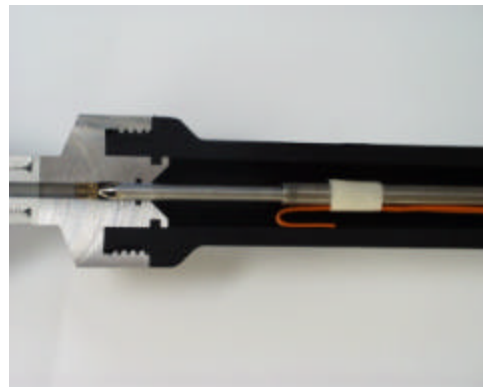
Fill stem & igniter wire inside a J motor
